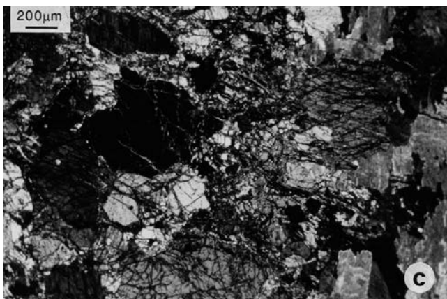
(a) shearing surfaces in serpentinites; (b) serpentinites (on the left) and harzburgite relic portions (top-right side) (crossed nicols, magnification x 25); (c) porphyroclastic texture of the harzburgite relic portions (crossed nicols, magnification x 25); (d) spinel-websterite lens in serpentinites (pencil length 15 cm.); (e) porphyroclastic texture of the spinel-websterite (crossed nicols, magnification x 25).
