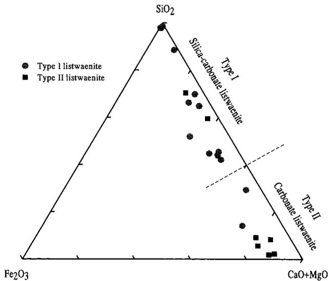
Fig. 5 - Plotting of listwaenites in SiO<sub>2</sub>-Fe<sub>2</sub>O<sub>3</sub>-CaO+MgO ternary diagram. Dashed line divides the silica-carbonate (type I) and carbonate (type II) listwaenites. Data are from Table 2.
