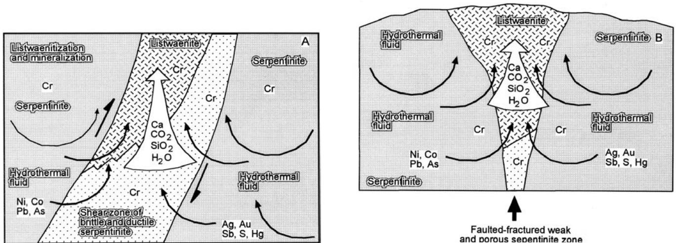
Fig. 9 - Suggested model for listwaenitization and mineralization in the Divriği-Hekimhan region. A) Thrust fault related model, B) Non-thrust fault related model. When carbonate listwaenite is subject to this model, silica is considered to be absent from the hydrothermal fluids (Uçurum, 1996).
